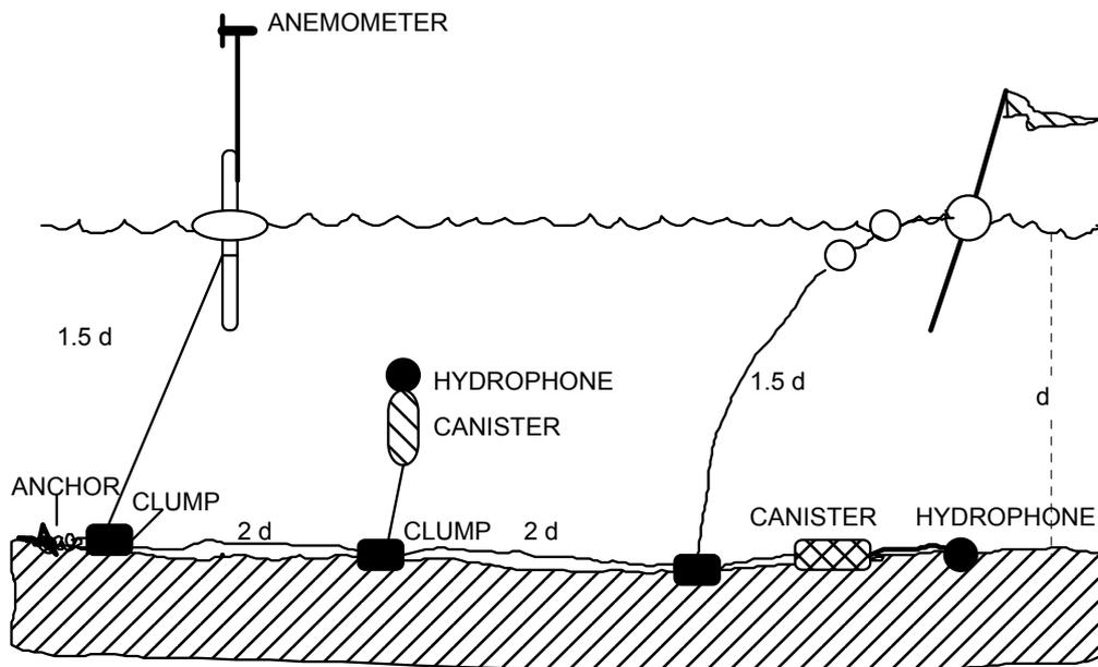
Figure 1: Ambient noise and wind recording system with hydrophone on the bottom and one buoyed up from the bottom. This is not to scale: anchors and line to hydrophone and canister should be far enough apart to ensure that the lines cannot tangle. Nominal line lengths in terms of the water depth  $d$  are shown.
